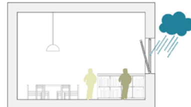
Figure 3 Illustrative drawing of protection against rain entry – Tilt window (Azevedo, 2012).
