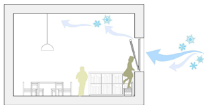
Figure 2 Illustrative drawing of ventilation impact on the occupation area – Tilt window (Azevedo, 2012).
